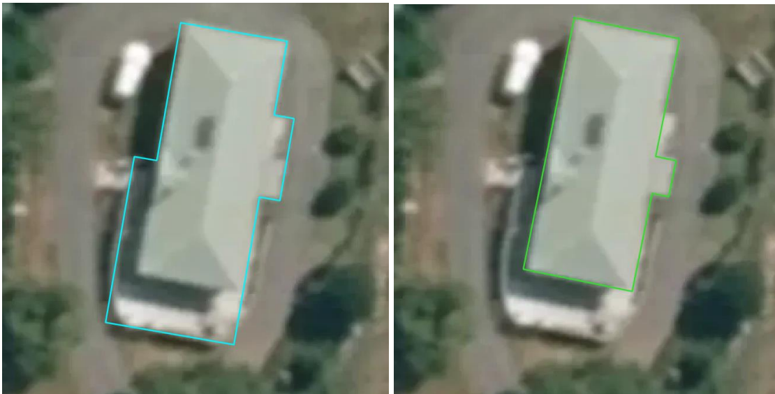
Incorrect capture of deck attached to building (left). Correct non-capture of deck (right).
