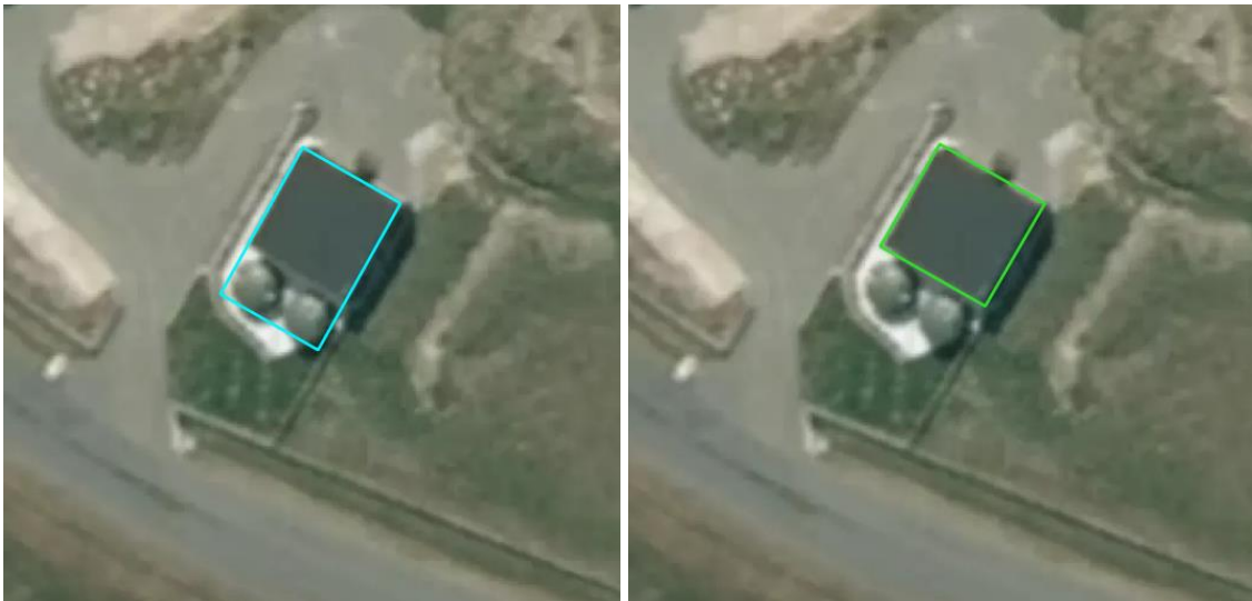
Incorrect capture of undersized tanks and grouping them with nearby building (left). Correct non-capture of undersized tanks (right).
