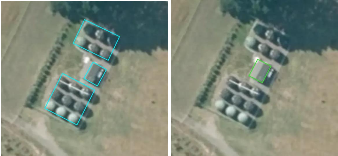
Incorrect capture and grouping of multiple undersized tanks (left). Correct non-capture of undersized tanks (right).
